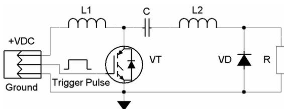
Figure 1. The DSRD current driver scheme
