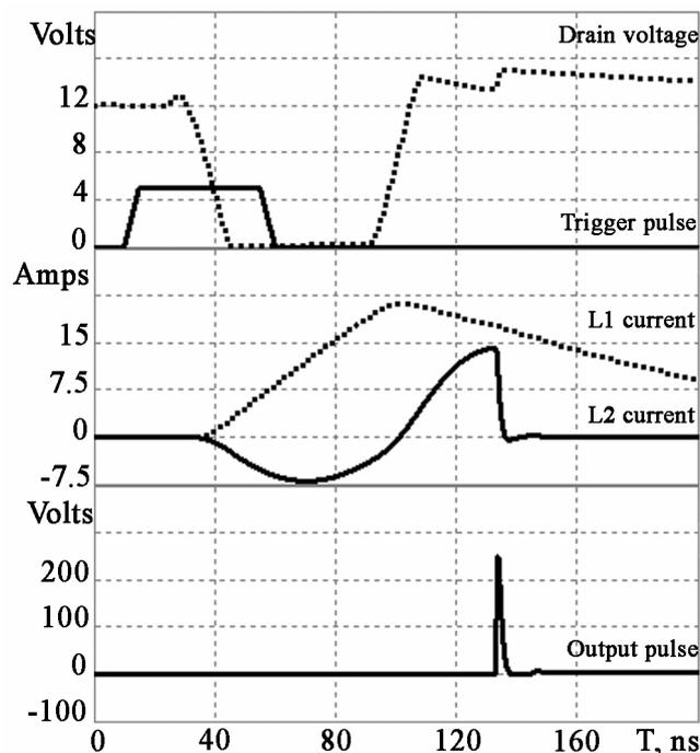
Figure 2. Waveforms of different points of the scheme: trigger pulse (a), MOSFET's drain voltage (b), current through L1 (c), current through L2 (d), load voltage (e).
