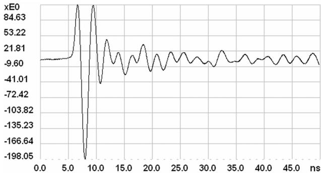
Figure 6. Receiving signal waveform on 4.5 meters distance between transmitter and receiver
