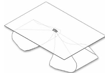
Figure 4. TEM horn with kinetic energy accumulation.
