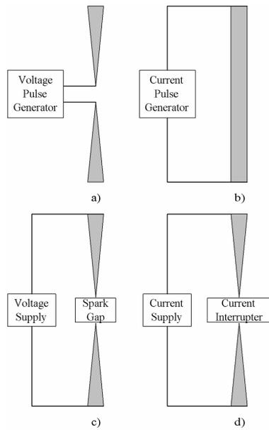
Figure 3. Antenna with voltage (a) and current (b) excitation, potential (c) and kinetic (d) energy accumulation.
