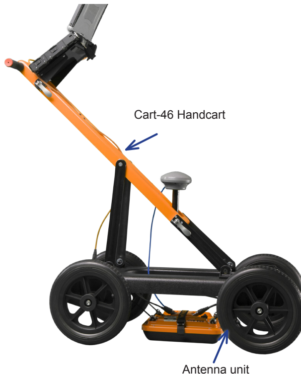
Antenna unit with Cart-46 Handcart
