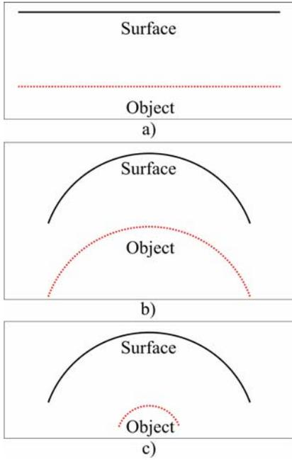
Figure 2. Topographic correction of the GPR profile: without correction (a), elevation correction (b), elevation and antenna tilt correction (c)
