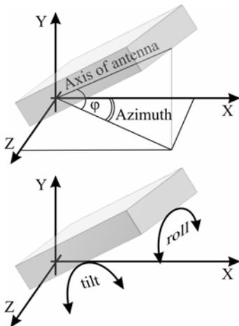
Figure 3. Orientation of the GPR antenna
