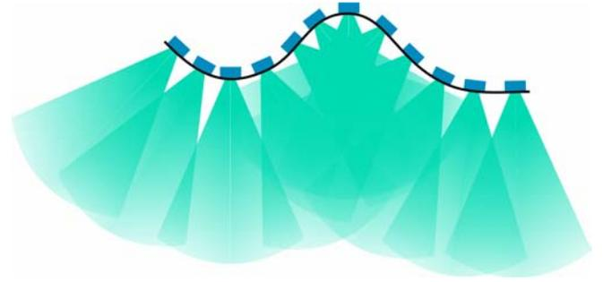
Figure 5. Topographic correction based on elevation, tilt and radiation pattern information
