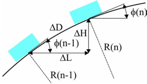
Figure 4. Movement along a curvilinear trajectory
