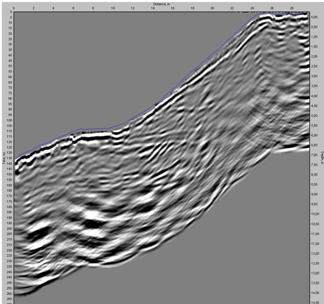
Figure 8. The GPR profile after topographic correction
